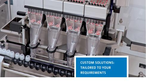
The 6-channel tablet and capsule counting modules do not require any format parts, are very easy to clean and free of calibration and extensive maintenance. All product contact parts are made from pharma grade materials and are suitable for autoclave cleaning. An optional cleaning trolley can be used for convenient cleaning and storage of the product contact parts. The slim design allows for a variable number of counting modules to be placed into the CFS-622 while maintaining a small footprint.
